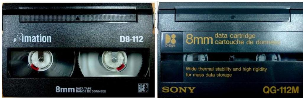
**Fig 02: 8mm (Exabyte) tape cartridges**
