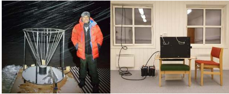
Figure 9.1: (L) Discone antenna placed on rooftop of Gruvebadet laboratory to sense electromagnetic signal in the frequency range 5 to 500 MHz; (R) Radio frequency interference recording system set up inside the Gruvebadet laboratory, Ny-Ålesund.
